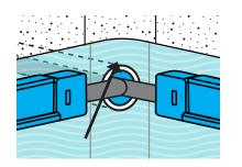
For concrete pools, seal conduit entry with pool-grade silicone sealant. *DO NOT drill holes in fiberglass pools/ hot tubs or vinyl-lined pools*. An alternate method is to route the wire directly out of pool.
