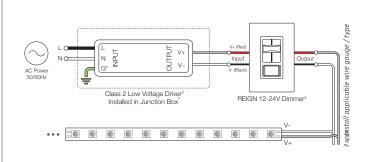
1. Driver may not require a fault ground connection. Refer to driver specifications for additional information.
